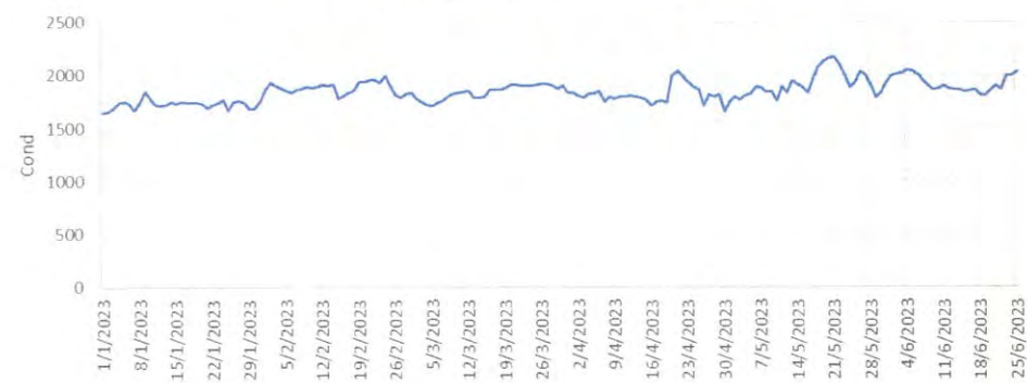
Conduct Cooling Water system side cracker
